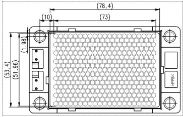
Dimension in mm, tolerance: ±1 mm
